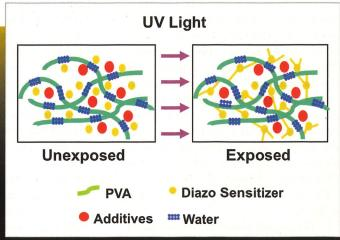
The image on the left illustrates the emulsion curing process as it is intended to occur. The image on the right shows how moisture in the emulsion coating impedes the curing process. Each shows the chemical structure of emulsion before and after exposing. Notice how the bonding sites between the diazo sensitizer and the polyvinyl alcohol (PVA) are inhibited by the water molecules in the emulsion coating, thus significantly weakening the stencil. (All images courtesy the author)
