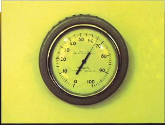
Using a hygrometer to measure and monitor relative humidity, shown here in a safelight protected screen drying room, is essential in all areas where coated screens are handled. With relative humidity at 65 percent, the hygrometer shows us this room is not properly controlled.
