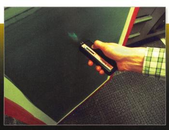
Moisture meters can be used to help determine when screens are dry enough to be exposed. Use the moisture meter again just before exposing to assure screens are still dry.
