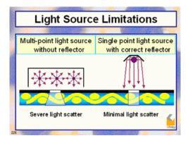
It is essential to use a lamp design that provides collimated light output which minimizes light scatter through a lamp design that directs the light straight onto the screen. Ask for the resolution of the lamp and ,make a few test screens before you purchase an expensive exposure system that promises high resolution but can not harden the emulsion to the correct level.
