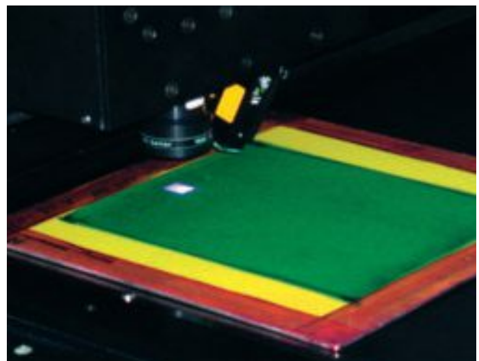
Figure 1 (left): DLP technology illustration. Figure 2 (right): Digital direct exposure system.
