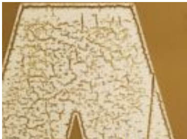
Figure 4: Image that has not been washed out properly.
