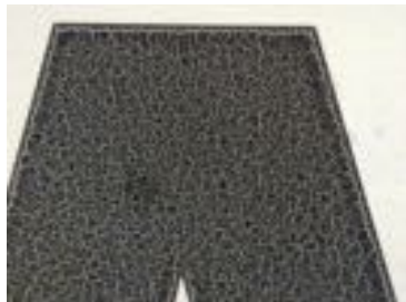
Figure 3: Crevasses resulting from incompatible surface tension.
