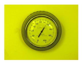
With relative humidity at 65%, the hygrometer shows us this room is not properly controlled.
