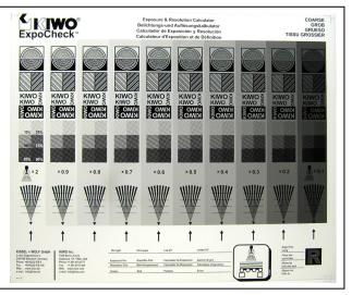
Determining the exposure time to use for the test exposure is key to using exposure calculators correctly. Use a *test* exposure time equal to two times the *expected* exposure. Expected exposure could be: the exposure times currently used, an estimate of the anticipated exposure based on experience, or exposure data obtained from the emulsion manufacturer.
