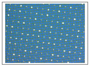
Another example below shows poor art-to-mesh relationship as it relates to text. In this example you see the letter F – although fully resolved by the emulsion – falls directly on a thread, while the letter L luckily falls in between the threads. This case illustrates how choosing the wrong mesh count also causes problems. The mesh count here is a 156-64, which clearly is unable to support this fine detail. This artwork requires a much finer mesh count.
