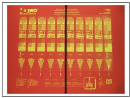
Each step has an associated number (as seen in the image below) that is used as the multiplier for calculating the representative exposure for that step. This number is multiplied by the time used to expose the calculator.
