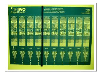
Therefore, the first exposure step left of the black line is considered to have received enough UV to provide very good chemical and mechanical resistance. This completes step one of the two-step process of determining proper stencil exposure.
