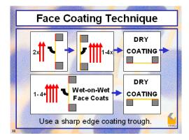
The fifth rule is: Use a combination of wet-on-wet and face coating techniques for a thin stencil with low Rz.
