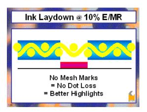
In this example, it is also quite likely the screen also suffered from an Rz value which was too high. Both high Rz and low EOM results from poor coating techniques. The poor gasket from the Rz allows the ink to leak into the valleys of the stencil. This results in dot gain. The 'sawtooth' from low EOM resulted in dot loss.
