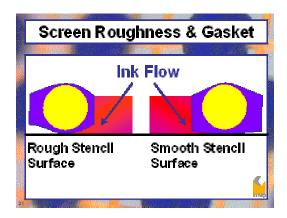
Perfect contact is achieved when both stencil and substrate are perfectly smooth. Poor contact is the result of rough substrate surfaces and rough stencil surfaces.
