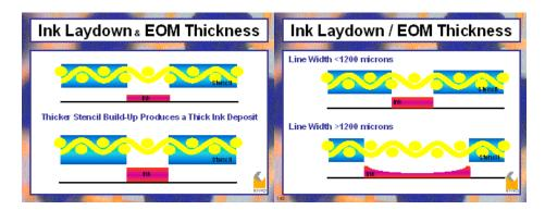
The ink laydown is determined by the 3-dimensional structure of the mesh, namely the mesh thickness and the mesh opening. These parameters determine the amount of ink the mesh can hold and hence transfer to the substrate.
