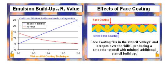
With this coating technique the stencil thickness can be adjusted micron by micron and a repeatability of plus or minus 1 micron can be achieved even when hand coating.
