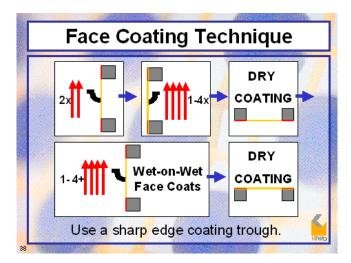
The second method of coating is face coatings or wet-on-dry coatings. Starting with a 1+1 wet-on-wet coat the mesh is filled with emulsion. After drying the screen several coats are applied to the substrate side of the screen with intermediate drying. This produces a thin, but very smooth coating and keeps the stencil thickness to a minimum.
