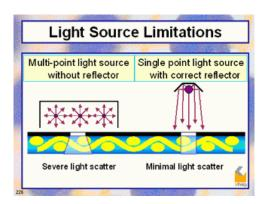
For optimum resolution use the thinnest possible mesh, dyed with yellow or orange color, coated with a dyed emulsion to the minimum emulsion build up of approximately 5 micron above mesh.
