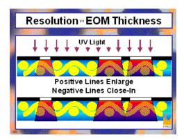
In many cases the exposure unit itself is limiting the maximum resolution due to poor lamp and reflector designs. The exposure unit should provide collimated light output.
