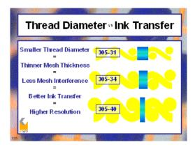
If possible, the finest line or the smallest dot should be as large as 2 mesh openings and 2 thread diameters combined or have a width twice the size of the total stencil thickness.
