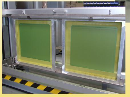
Suitable for coating one screen with a maximum single frame size of 53" X 53" (137 cm x 137 cm) outside dimensions or two screens with maximum single frame sizes of 25" X 53" (63 cm x 137 cm) outside dimensions. A Coating trough pin registration system that allows for 1-up or 2-up coating comes standard with each machine.
