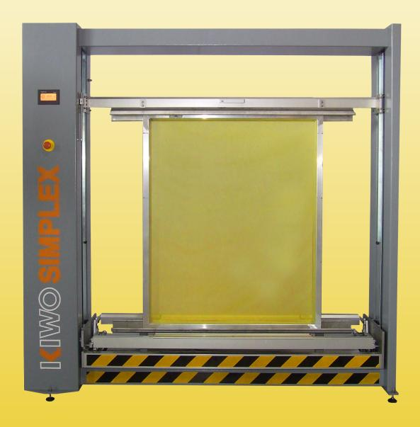
The KIWO SIMPLEX<sup>(TM)</sup> Screen Coating Machine is specifically designed for textile and small graphic applications, providing superior performance at a budget price. Manufactured by Grunig for KIWO it offers reliable coating results within close tolerances.
