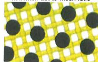
Film on mesh showing minimum dot-to-mesh ratio
