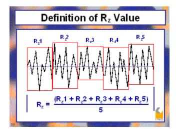
To obtain the sharpest printed image, a roughness (Rz) value of less than 10 microns is desirable for the stencil. More specifically, when combining the Rz value of the stencil and the Rz of the substrate, a value of 12 to 15 microns or less is ideal. If the Rz value is higher or the stencil rougher, the ink is likely to flow underneath the stencil edge, causing saw-toothing and smearing the print.
