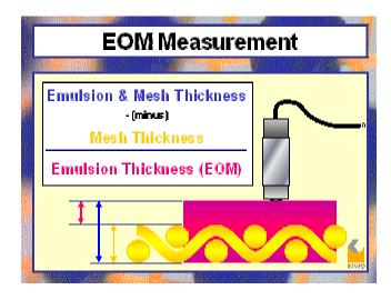
The following applies to both rules: If the emulsion coating is too thin, it will not provide a proper gasket seal. The ink will bleed underneath the stencil. This will cause the print to have rough looking edges (saw-toothing). Other symptoms of inadequate emulsion thickness include smeared images, dot loss in the highlights and dot gain in the shadows.
